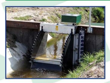
Panel Stainless steel box in which all components are housed
